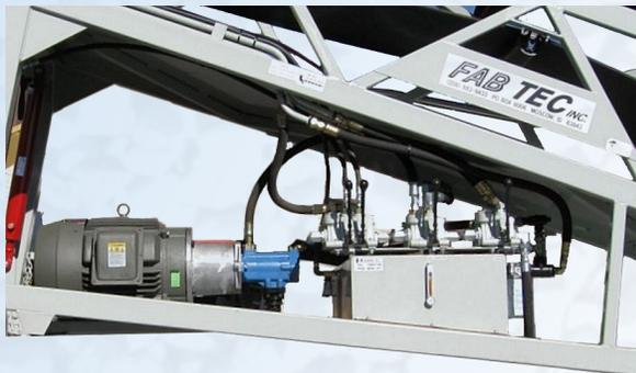
40 HP TEFC motor ~vs~ Deutz diesel to run the hydraulic pump.
