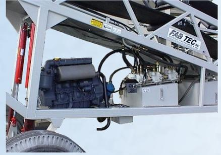
Deutz F4L2011 air cooled diesel has 55 hp at 2100 rpm
